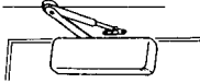
FIGURE 11.77 Door-closer spring closes the door, while a hydraulic mechanism (cylinder with piston) keeps the door from slamming.
