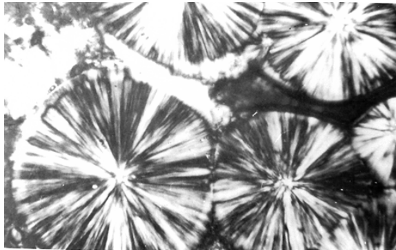
Figure 4.5 An optical micrograph of PP Spherulites
