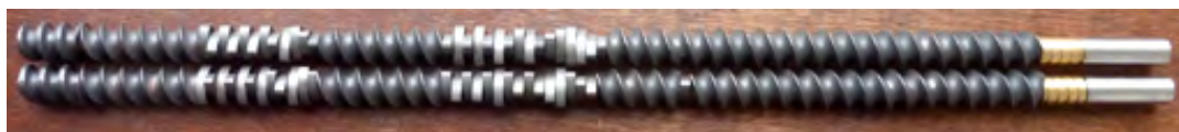
Figure 3.24 Conveyor elements and kneading disks are assembled on the shafts of twin screws
