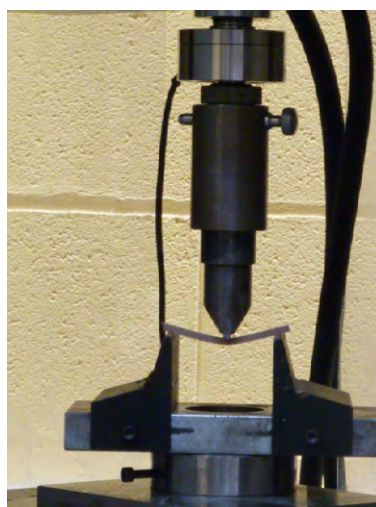
Figure 6.14 A specimen tested in 3-point bending
