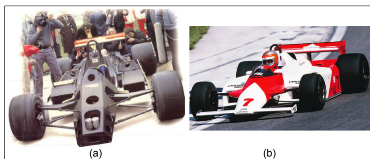
Figure 5.19 The first carbon-fibre composite Grand Prix car: (a) monocoque McLaren MP4/1 (1980); (b) McLaren MP4 (MP4/1) competed in the 1981 Formula One Season (sources: Savage 2008, p. 11, and F1Technical.net)
