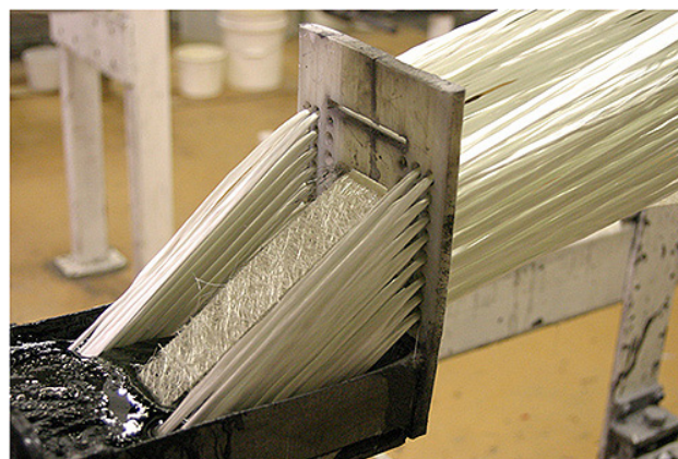
Figure 2.14 Open-bath pultrusion forming (source: Martin Pultrusion)
