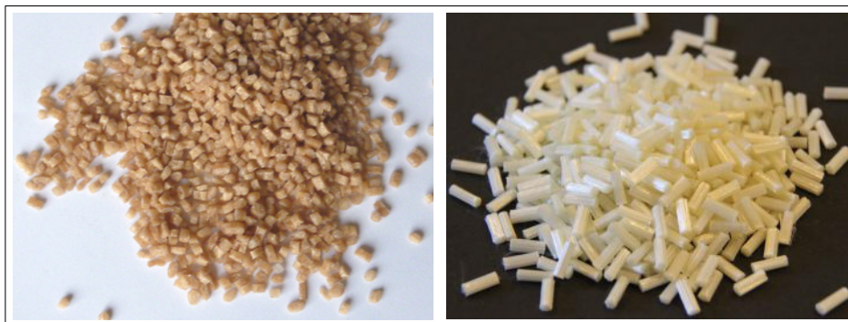
Figure 2.22 Granules/pellets of SFT and LFT
