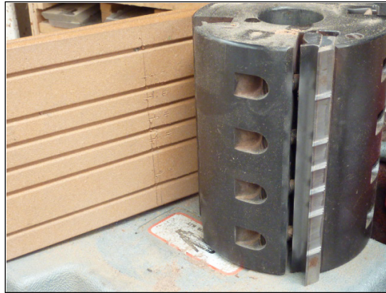
Figure 2.30 The rotary profile/moulding cutter
