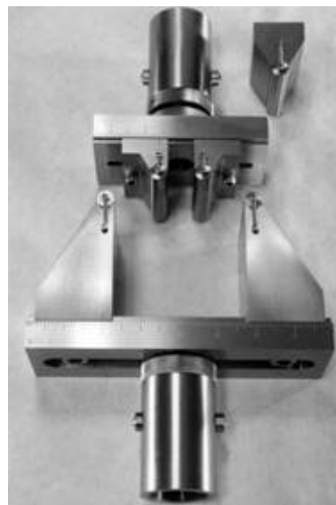
Figure 4.5 Three and four-point flexure test fixtures (note that with this setup the upper adapter is connected to 4-point loading head) (source: Wyoming Test Fixtures)
