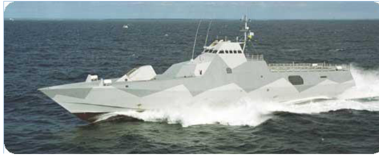
Figure 5.20 Swedish Navy Visby stealth corvette: 600 tons – 72 m long – FRP sandwich (source: Wikipedia 2014)
