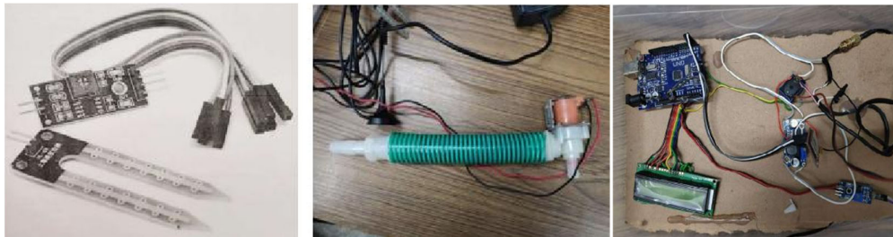
Moisture detection sensor, connector with value and relay control, and LCD display with control and communication devices
